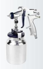
Standard Nozzle: 1.8mm Optional Nozzle: 1.5-2.0mm Operating Pressure: 50-70psi Pattern Width: 110-280mm Air Consumption: 7.5cfm Cup Capacity: 1000ml
