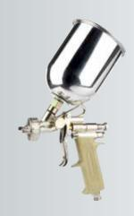
Standard Nozzle: 1.5mm Optional Nozzle: 1.5-2.0mm Operating Pressure: 50-70psi Pattern Width: 110-280mm Air Consumption: 7.5cfm Cup Capacity: 600ml Measure: 66x32x41.5cm/10pcs Weight: 22/20kg
