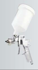
Standard Nozzle: 1.5mm Optional Nozzle: 1.2-2.0mm Operating Pressure: 50-70psi Pattern Width: 110-250mm Air Consumption: 11.5cfm Cup Capacity: 600ml Measure: 67.5x47x26.5cm/20pcs Weight: 18/16kg
