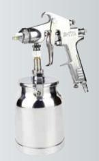
Standard Nozzle: 1.5mm Optional Nozzle: 1.3-2.5mm Operating Pressure: 50-70psi Pattern Width: 200-240mm Air Consumption: 7.2cfm Cup Capacity: 1000ml Measure: 61.5x37.5x25.5cm/10pcs Weight: 13/12kg
