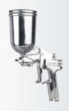
Standard Nozzle: 1.5mm Optional Nozzle: 1.0-2.0mm Operating Pressure: 50-70psi Pattern Width: 150-250mm Air Consumption: 11.5cfm Cup Capacity: 400ml
