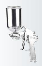
Standard Nozzle: 1.5mm Optional Nozzle: 1.0-2.0mm Operating Pressure: 50-70psi Pattern Width: 150-250mm Air Consumption: 11.5cfm Cup Capacity: 400ml Measure: 54.5x40.5x25cm/20pcs Weight: 18/16kg
