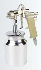
Standard Nozzle: 1.5mm Optional Nozzle: 1.5-2.0mm Operating Pressure: 50-70psi Pattern Width: 110-280mm Air Consumption: 7.5cfm Cup Capacity: 1000ml Measure: 57.5x38x28.5cm/10pcs Weight: 10/9kg
