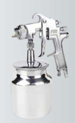
Standard Nozzle: 1.5mm Optional Nozzle: 1.5-2.0mm Operating Pressure: 50-70psi Pattern Width: 180-250mm Air Consumption: 8.3cfm Cup Capacity: 750ml Measure: 57.5x35x28.5cm/10pcs Weight: 19/17kg
