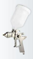
Standard Nozzle: 1.4mm Optional Nozzle: 1.2-2.5mm Operating Pressure: 50-70psi Pattern Width: 180-240mm Air Consumption: 8.8cfm Cup Capacity: 600ml Measure: 66.5x24.5x26.5cm/10pcs Weight: 13/12kg
