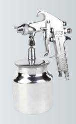
Standard Nozzle: 1.5mm Optional Nozzle: 1.3-2.5mm Operating Pressure: 50-70psi Pattern Width: 180-240mm Air Consumption: 11.2cfm Cup Capacity: 750ml Measure: 67x43x26.5cm/10pcs Weight: 19/17kg
