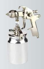
Standard Nozzle: 1.5mm Optional Nozzle: 1.0-2.0mm Operating Pressure: 50-70psi Pattern Width: 110-250mm Air Consumption: 11.2cfm Cup Capacity: 1000ml Measure: 52.5x26x30.5cm/6pcs Weight: 9/7kg
