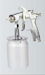
Standard Nozzle: 1.5mm Operating Pressure: 50psi Pattern Width: 150mm Air Consumption: 4cfm Cup Capacity: 600ml
