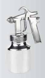
Standard Nozzle: 1.3mm Optional Nozzle: 1.5-2.5mm Operating Pressure: 50psi Pattern Width: 170mm Air Consumption: 4cfm Cup Capacity: 1000ml Measure: 57.5x38.5x31cm/10pcs Weight: 11/10kg
