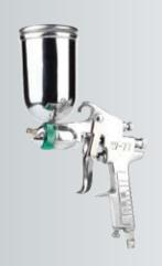
Standard Nozzle: 2.0mm Optional Nozzle: 1.5-3.0mm Operating Pressure: 50-70psi Pattern Width: 120-250mm Air Consumption: 10.5cfm Cup Capacity: 400ml Measure: 44.5x35x23cm/10pcs Weight: 10/9kg
