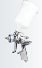
Standard Nozzle: 1.5mm Optional Nozzle: 1.0-2.2mm Operating Pressure: 50-70psi Pattern Width: 110-280mm Air Consumption: 7.5cfm Cup Capacity: 600ml
