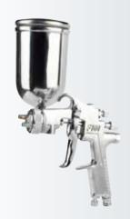
Standard Nozzle: 1.5mm Optional Nozzle: 1.5-2.0mm Operating Pressure: 50-70psi Pattern Width: 180-250mm Air Consumption: 8.3cfm Cup Capacity: 400ml Measure: 51.5x41.5x28.5cm/10pcs Weight: 18/16kg
