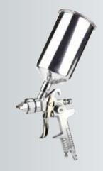
Standard Nozzle: 1.4mm Optional Nozzle: 1.2-2.5mm Operating Pressure: 20-50psi Pattern Width: 190mm Air Consumption: 7.5cfm Cup Capacity: 1000ml Measure: 63x48x24.5cm/10pcs Weight: 13/12kg
