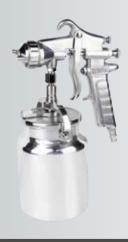
Standard Nozzle: 1.0mm Optional Nozzle: 1.0-2.0mm Operating Pressure: 50-70psi Pattern Width: 150mm Air Consumption: 14.5cfm Cup Capacity: 1000ml Measure: 69.5x32.5x26cm/10pcs Weight: 11/10kg
