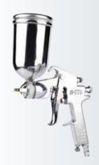
Standard Nozzle: 1.5mm Optional Nozzle: 1.3-2.5mm Operating Pressure: 50-70psi Pattern Width: 200-240mm Air Consumption: 7.2cfm Cup Capacity: 400ml Measure: 61.5x37.5x25.5cm/10pcs Weight: 10/9kg
