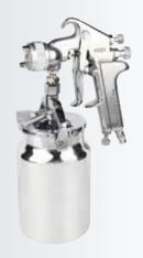
Standard Nozzle: 1.8mm Optional Nozzle: 1.4-2.5mm Operating Pressure: 65-90psi Pattern Width: 280mm Air Consumption: 14cfm Cup Capacity: 1000ml Measure: 54x38x32cm/10pcs Weight: 14/12kg
