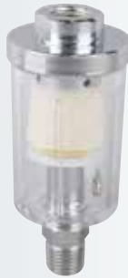
AFR-81-1 Air Filter - Pipe Size: 1/4" - Use Pressure: 6bar - Endure Pressure: 8bar - Working Pressure: 0-6bar - Packing: colour box
