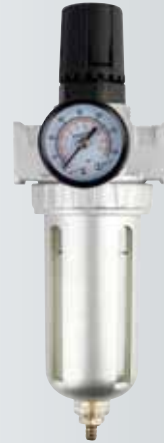
AFR-80-02 Air Filter Regulator - Pipe Size: 1/4", 1/2", 3/8" - Use Pressure: 10bar - Endure Pressure: 15bar - Working Pressure: 0-7bar - Packing: colour box - G.W./N.W: 15/14kgs 25pcs/CTN - Measure: 48x47.5x21cm
